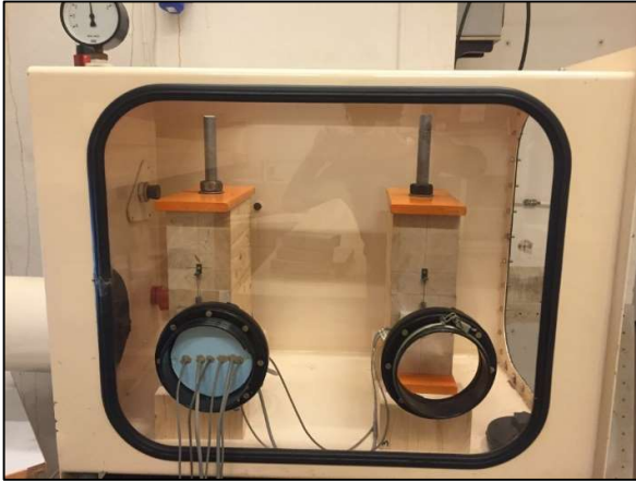
Figure 4: Specimens and setup into the sealed climate-controlled chamber.
