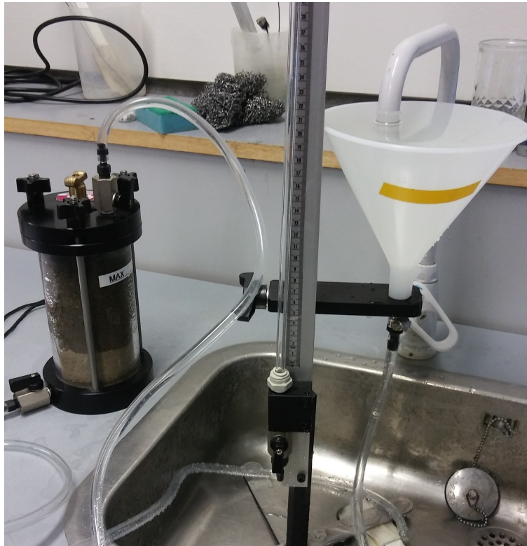
Figure 3.1: Permeameter cell used for initial testing
