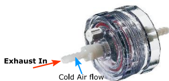
Figure 9. 47mm polycarbonate inline filter holder. Plastic hose spears were replaced with stainless Swagelok items. Filters used were 2500 QAT-UP 47mm.
