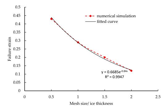
Figure 11. Relationship between failure strain and size ratio.
