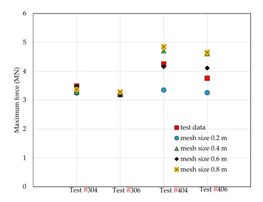
**Figure B1.** Comparison of the maximum ice force between the simulated and measured results for all tests.
