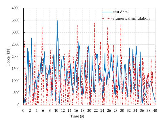
**Figure A4.** Ice force histories from the simulation with mesh size of 0.8 m and measurement for test #304.
