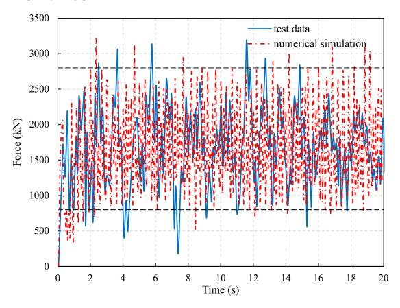
**Figure 12.** Ice force histories from the simulation with mesh size of 0.2 m and measurement for test #306.
