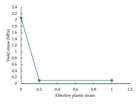
Figure 5. Hardening curve for ice material model.
