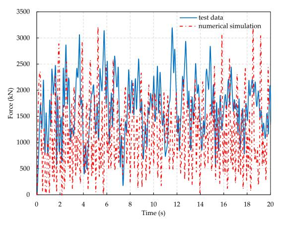
**Figure 13.** Ice force histories from the simulation with mesh size of 0.4 m and measurement for test #306.
