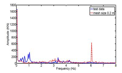
**Figure 19.** Spectrum of ice force from the simulation with mesh size of 0.2 m and measurement for test #306.
