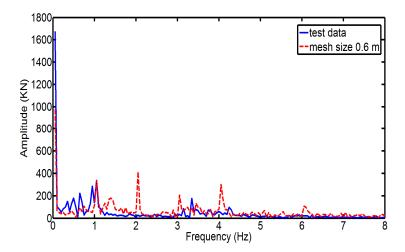
**Figure 21.** Spectrum of ice force from the simulation with mesh size of 0.6 m and measurement for test #306.
