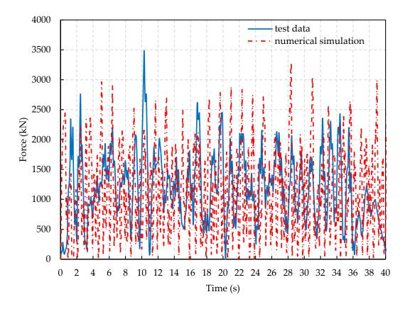
**Figure A2.** Ice force histories from the simulation with mesh size of 0.4 m and measurement for test #304.
