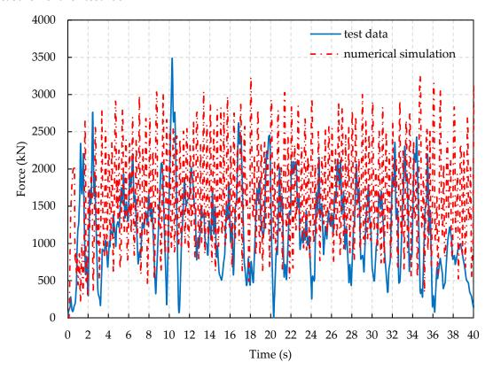
**Figure A1.** Ice force histories from the simulation with mesh size of 0.2 m and measurement for test #304.
