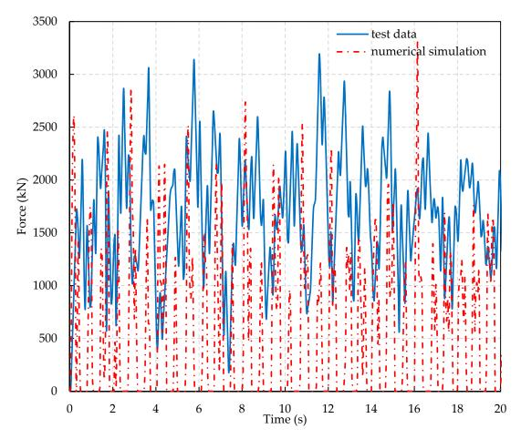
**Figure 15.** Ice force histories from the simulation with mesh size of 0.8 m and measurement for test #306.
