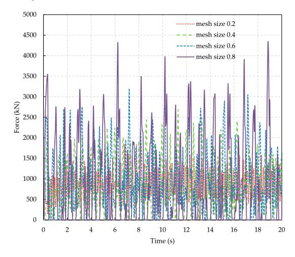
Figure 7. Ice force histories from the simulations with different mesh sizes.
