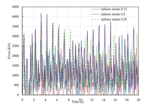
Figure 9. Ice force histories from the simulations with different failure strains.
