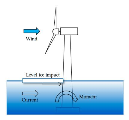
Figure 1. OWT exposed to wind field and in contact with ice.
