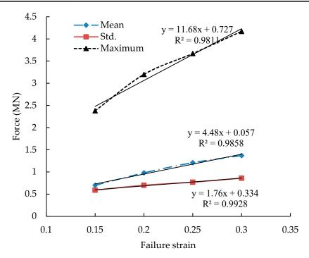
Figure 10. The mean, standard deviation, and maximum forces varying with the failure strain.
