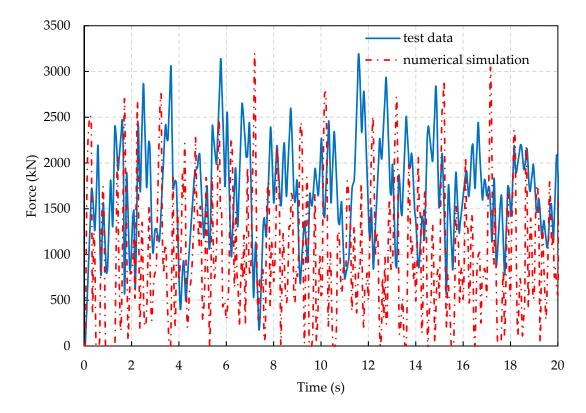
**Figure 14.** Ice force histories from the simulation with mesh size of 0.6 m and measurement for test #306.
