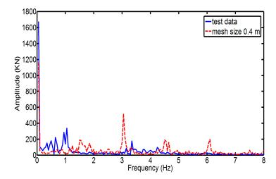
**Figure 20.** Spectrum of ice force from the simulation with mesh size of 0.4 m and measurement for test #306.
