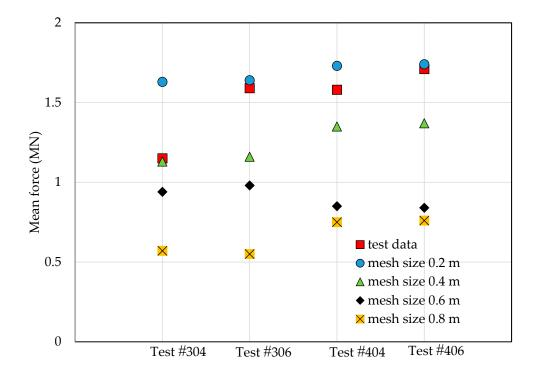
**Figure B2.** Comparison of the mean ice force between the simulated and measured results for all tests.
