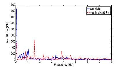
**Figure 22.** Spectrum of ice force from the simulation with mesh size of 0.8 m and measurement for test #306.
