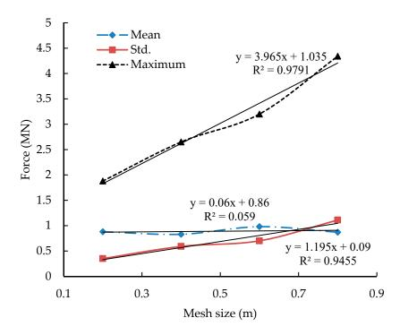
Figure 8. The mean, std. and maximum forces varying with the mesh size.
