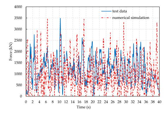
**Figure A3.** Ice force histories from the simulation with mesh size of 0.6 m and measurement for test #304.
