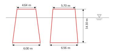
Figure 2. The geometry of the 3-MW and 4-MW wind turbine towers in full scale.
