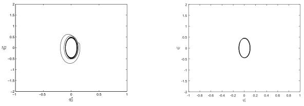
(a) Voltage-driven reference trajectory on  $(q_2^*,\dot{q}_2^*)\text{-plane}.$ (b) Torque-driven reference trajectory on  $(q_2^*, \dot{q}_2^*)$ -plane.
