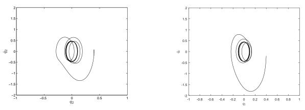
(a) Voltage-driven pendulum motion on  $(q_2, \dot{q}_2)$ -plane.
