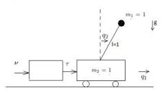
Figure 1.: Cart-pendulum model
