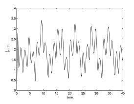
(a) Tracking error  $||(e_{p_1},e_{p_2},\dot{e}_{p_1},\dot{e}_{p_2})^T||_2$  for the voltage-driven plant.
