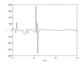
(b) Control input, computed for the torque-driven model and affected by actuator dynamics.
