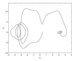
(a) Torque-driven pendulum motion on  $(q_2, \dot{q}_2)$ -plane, affected by actuator dynamics.
