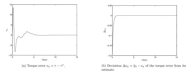
Figure 7.: Torque tracking error and its estimate for the disturbance-free voltage-driven plant.
