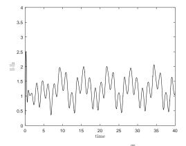
(b) Tracking error  $||(e_{p_1}, e_{p_2}, \dot{e}_{p_1}, \dot{e}_{p_2})^T||_2$  for the torquedriven plant.
