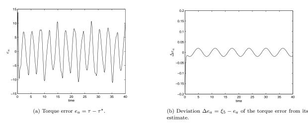
Figure 12.: Torque tracking error and its estimate for the voltage-driven plant in the presence of disturbances.
