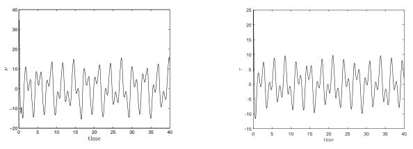
(a) Control input for the voltage-driven plant. (b) Control input for the torque-driven plant. Figure 11.: Control inputs  $\nu$  and  $\tau$  in the presence of disturbances.
