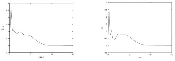
(a) Tracking error  $||(e_{p_1}, e_{p_2}, \dot{e}_{p_1}, \dot{e}_{p_2})^T||_2$  for the voltagedriven plant.
