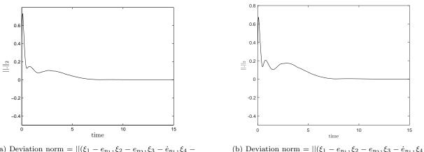
(a) Deviation norm =  $||(\xi_1 - e_{p_1}, \xi_2 - e_{p_2}, \xi_3 - \dot{e}_{p_1}, \xi_4 - \dot{e}_{p_2})^T||_2$  for the voltage-driven plant.
