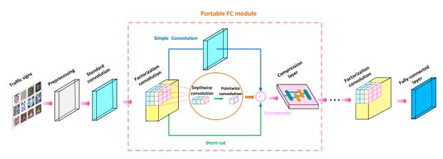
Fig. 1: Portable CNN Model consists of factorization convolution layers and compression layers.
