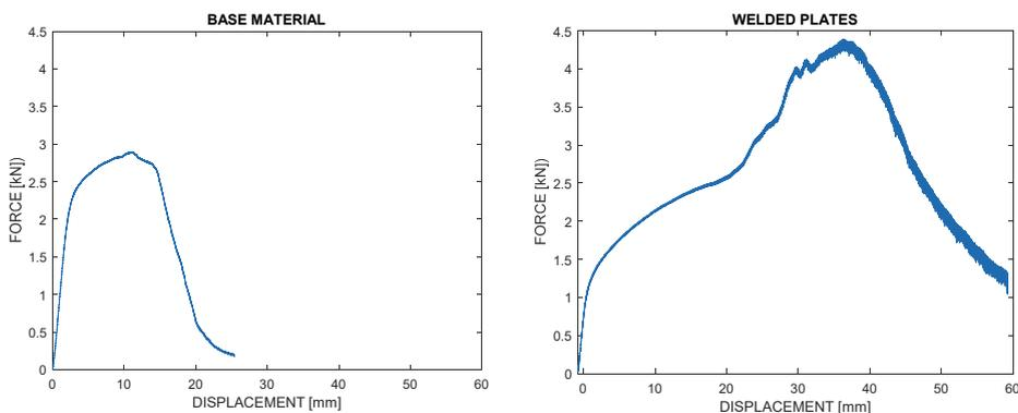
Figure 4: Force applied with the plunger on the Parent material (on the left) and on the welding (on the right).
