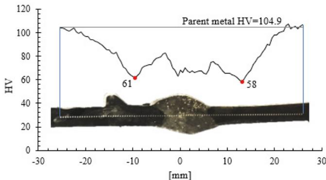
Figure 2: Hardness profile for the GMA weldment, including a macro image of the hardness specimen. The horizontal line at 104.9 represents the HV average value measured on the Parent Metal. The parent metal HV has a standard deviation of 1.7.
