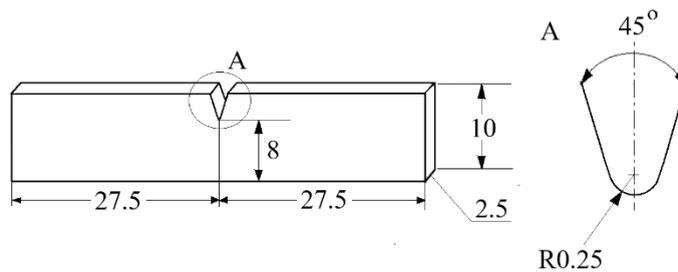
Figure 5: Geometry of the Charpy specimens tested.
