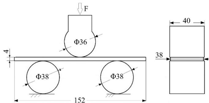
Figure 3: Bend test set-up.
