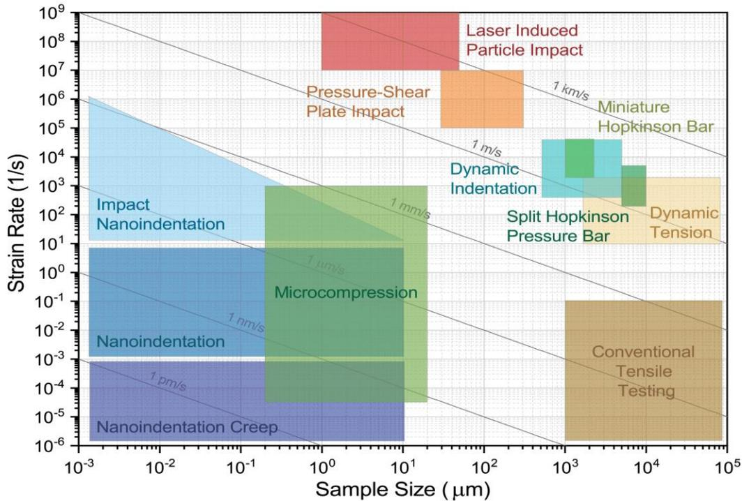
**Figure 2 – Schematic strain rate and sample length scale relationships for various mechanical testing techniques (19–26).**
