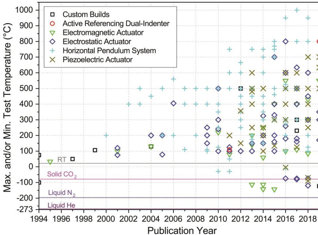
**Figure 1 - Maximum and/or minimum published small scale mechanical testing temperatures for various system configurations in recent years (14) - updated from (15).**
