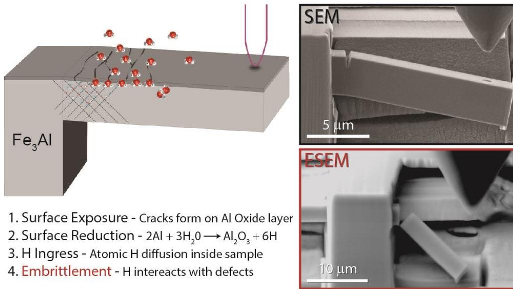
**Figure 3 – Schematic showing hydrogen ingress and embrittlement of a FeAl sample with *in situ* secondary electron micrographs showing the relatively tough behavior in vacuum in contrast with the hydrogen embrittled behavior in the ESEM (45).**
