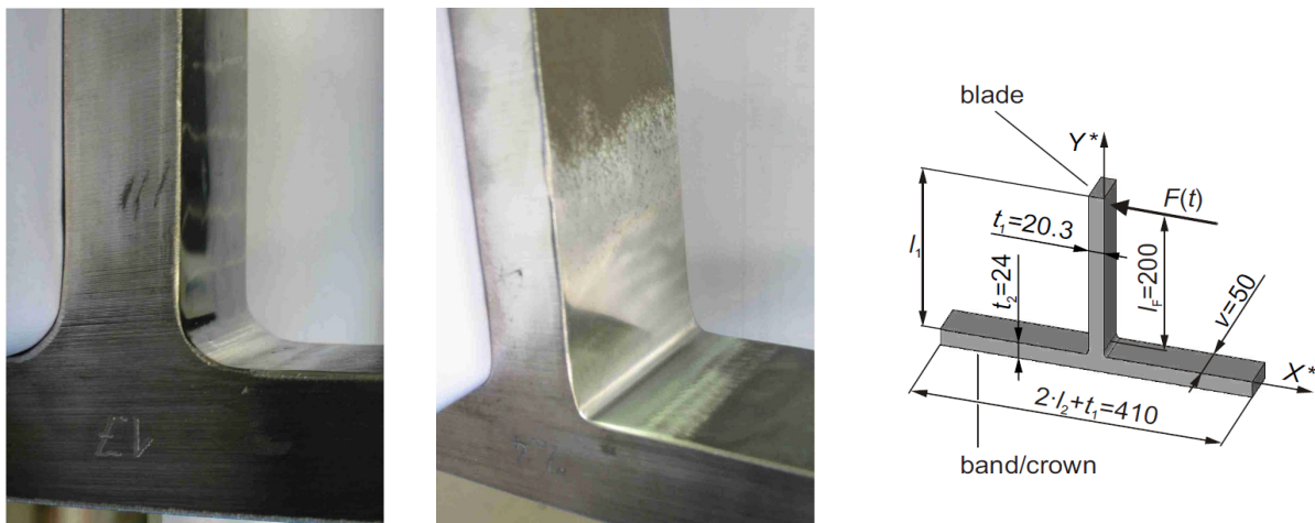
Figure 4: Specimens for bending tests under fatigue loading conditions from the literature [23]
