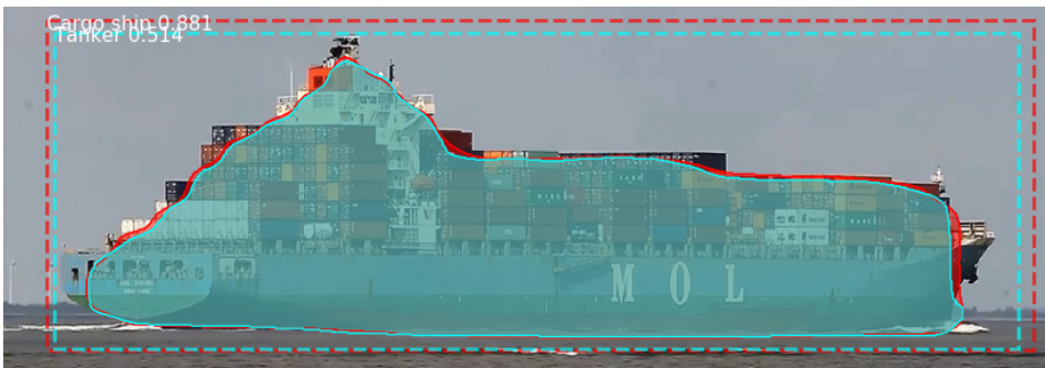
Figure 5.11: Overlapping detections of a real-world cargo ship. The detection with label "Tanker" would be removed since it has the lowest detection confidence.
