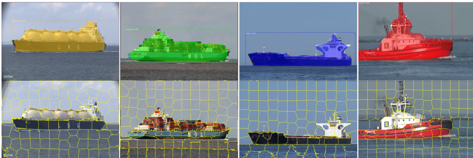
Figure 5.15: Original detection and super-pixel segmentation of images in the second LIME experiment. LNG carrier: 88 segments. Cargo ship: 100 segments. Tanker: 92 segments. Tugboat: 104 segments.
