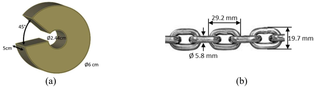
Figure 5. Geometry of (a) Buoyancy modules and (b) Ballast.
