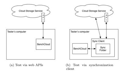
Figure 3.2: Two styles of test architecture
