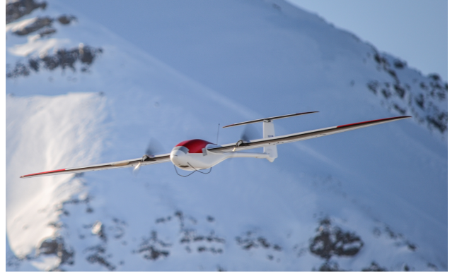
Figure 3: The NTNU Cruiser-Mini fixed-wing UAV with the thermal camera visible near the front.
