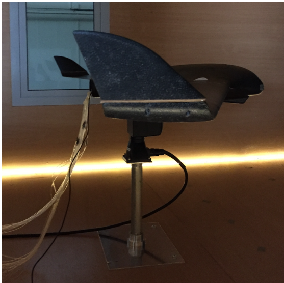
Fig. 5: A sideways view of the wind tunnel setup with the Skywalker X8 mounted on the PTU-D48.
