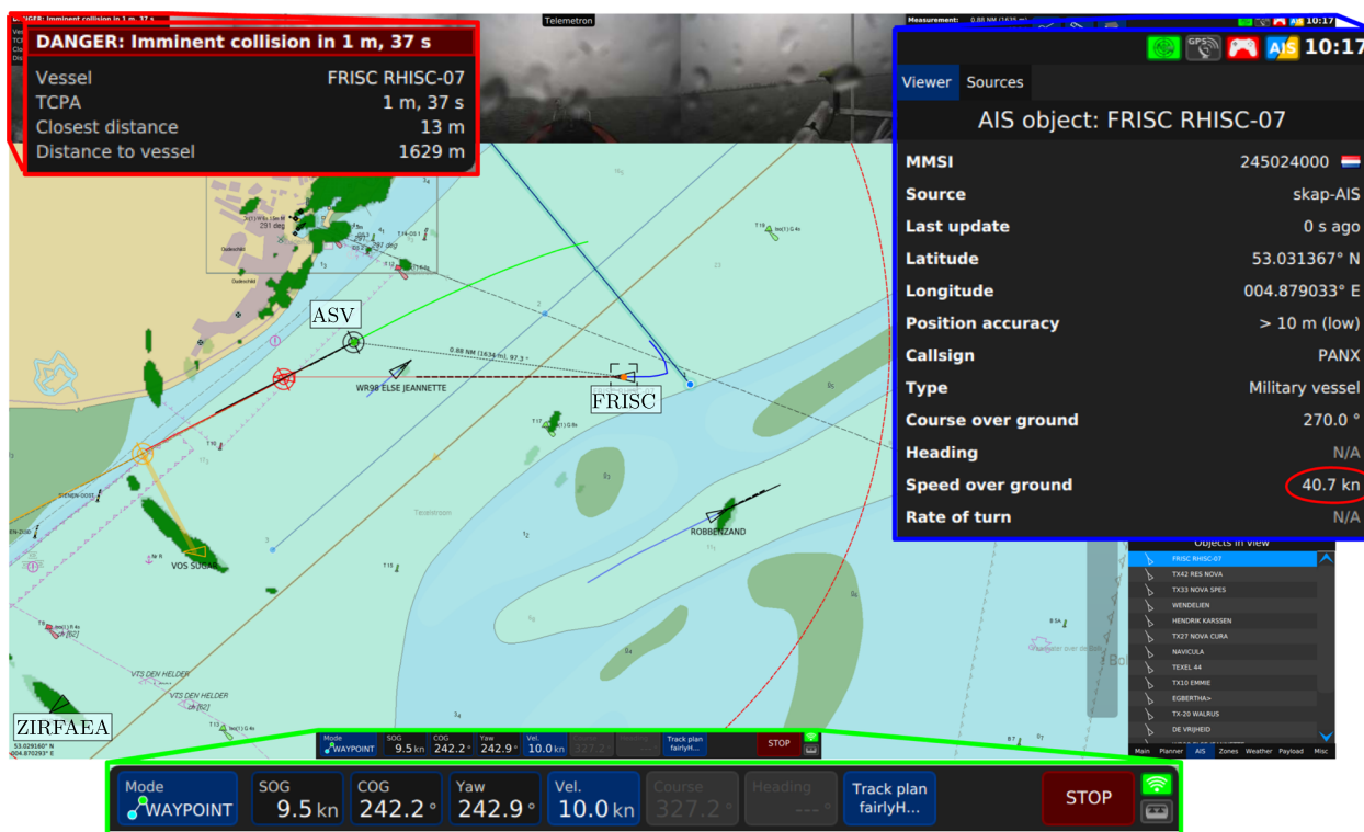
FIGURE 6 Vehicle control station (VCS) view showing information about the ASV (green bottom zoom window), obstacle vessel (blue upper right zoom window), and collision danger (red upper left zoom window). A prediction of the potential collision point between the ASV and FRISC is indicated with a red projection symbol, and a yellow projection indicates the CPA to another danger ahead. The large red arc is part of a circular collision avoidance region (of radius 1 NM) specified around the ASV. Obstacle vessels outside this region are not considered in the ASV's autonomous decision process. The solid blue and brown lines are planned paths tracked by the ASV (Telemetron), FRISC, or ZIRFAEA in different scenarios. ASV, autonomous surface vehicle; CPA, closest point of approach; FRISC, Fast Raiding, Interception and Special forces Craft [Color figure can be viewed at wileyonlinelibrary.com]
