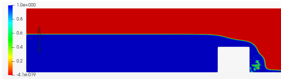
Figure 3-11 Numerical free water surface profile over a broad-crested weir by RNG K- \epsilon turbulence model
