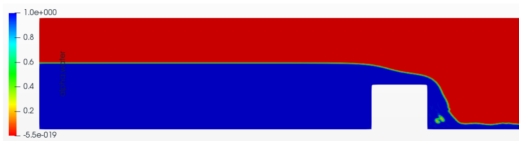
Figure 3-9 Numerical free water surface profile over a broad-crested weir by KomegaSST turbulence model
