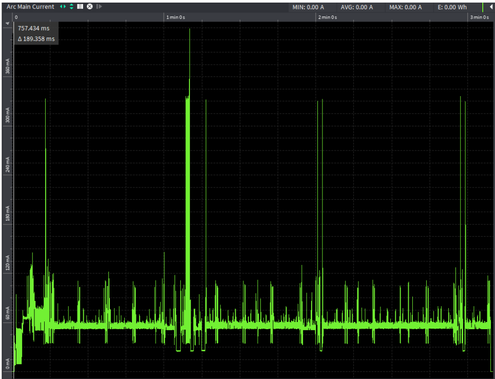
Figure 4.2: The first energy measurement on an NB-IoT transmission scheme
