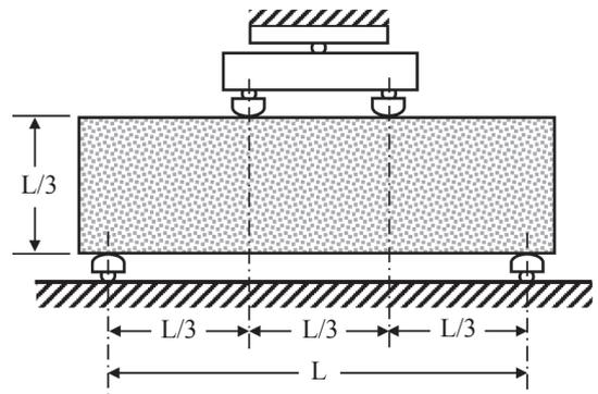
Fig. 4. Schematic view of bending test configuration (L = 15 mm).
