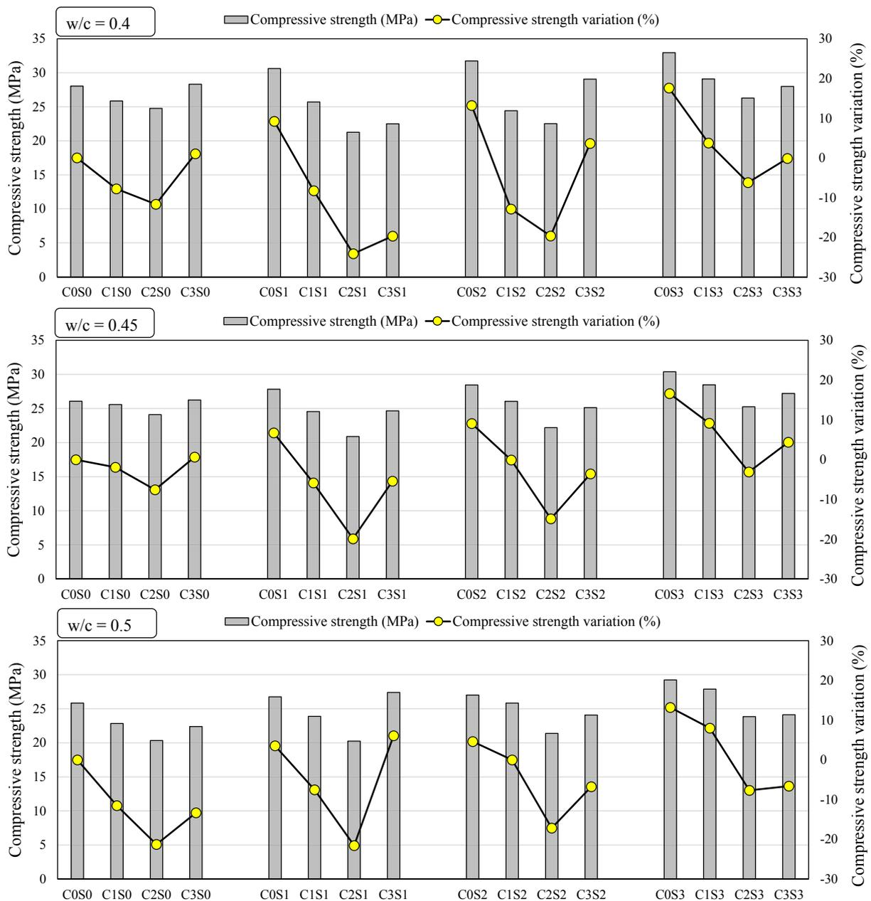
Fig. 3. Compressive strength values obtained for the modified concrete specimens with different amounts of nano additives and using different water to cement ratios.
