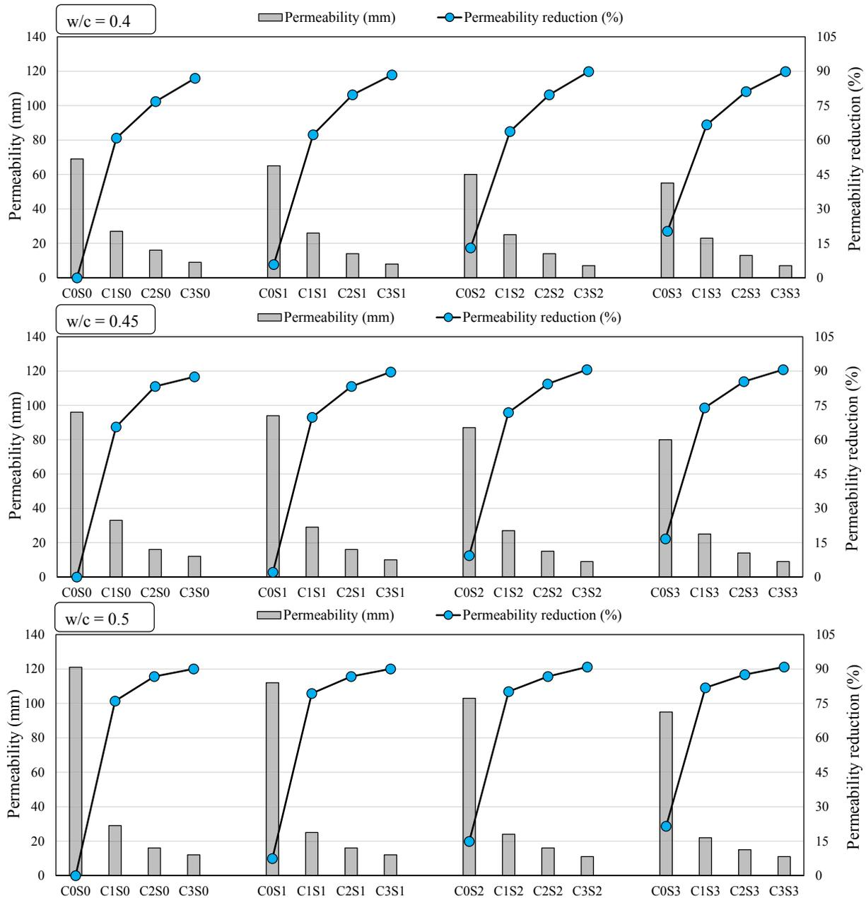
Fig. 7. Permeability values obtained for the modified concrete specimens with different amounts of nano additives and using different water to cement ratios.
