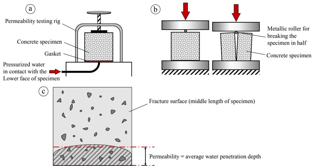
**Fig. 6.** Schematic view of permeability test; (a) concrete specimen in contact with pressurized water in a testing rig, (b) Breaking the test specimen into half in order to check the permeability, (c) obtaining the average length of the moist concrete from the fracture surface.
