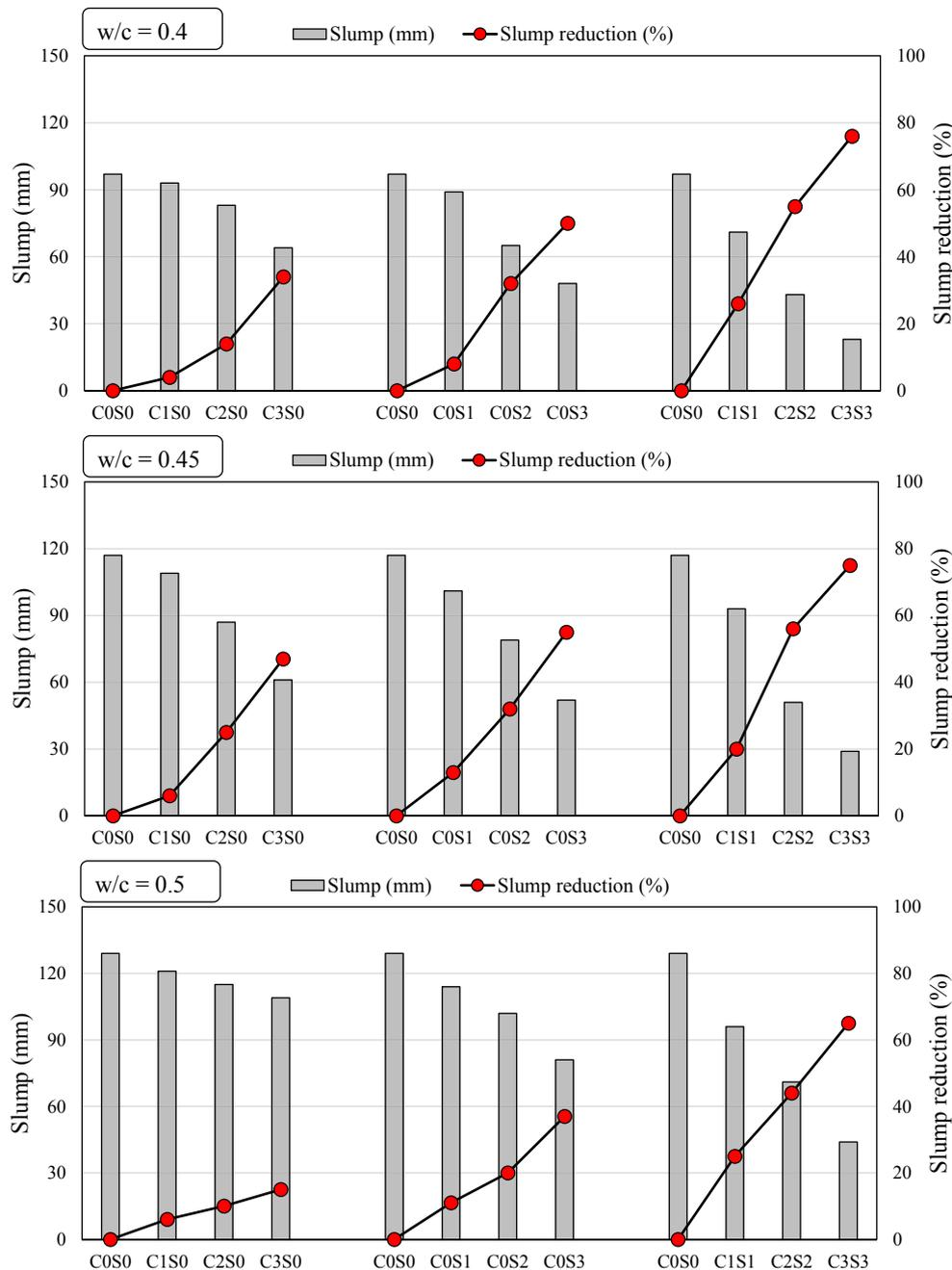
Fig. 2. The amount of slump and the amount of slump reduction based on the percentage of nano-particles for different w/c values.
