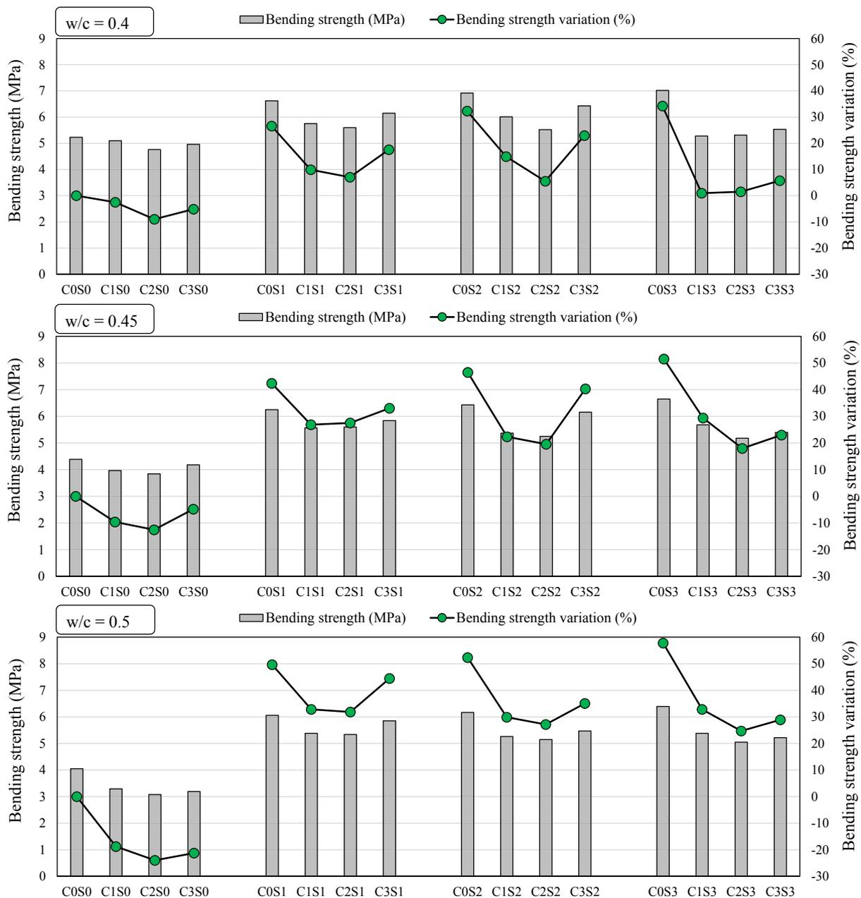
Fig. 5. Bending strength values obtained for the modified concrete specimens with different amounts of nano additives and using different water to cement ratios.
