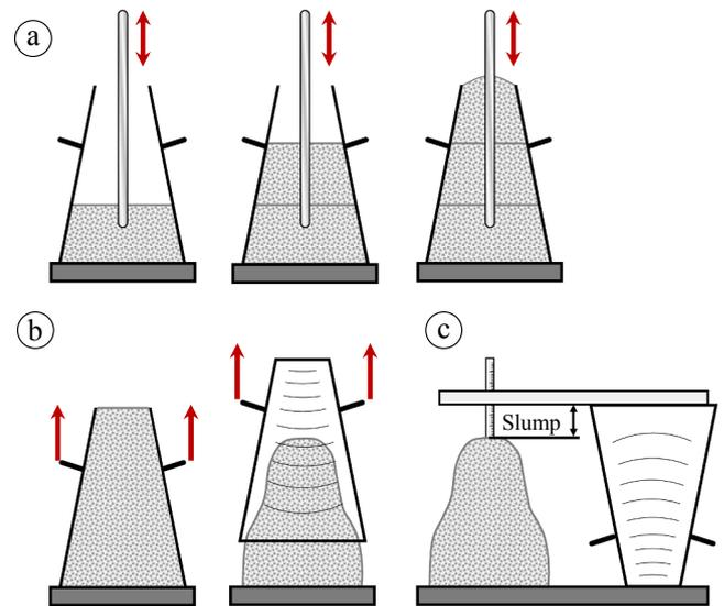
**Fig. 1.** Schematic view of slump testing of the concrete mixture.
