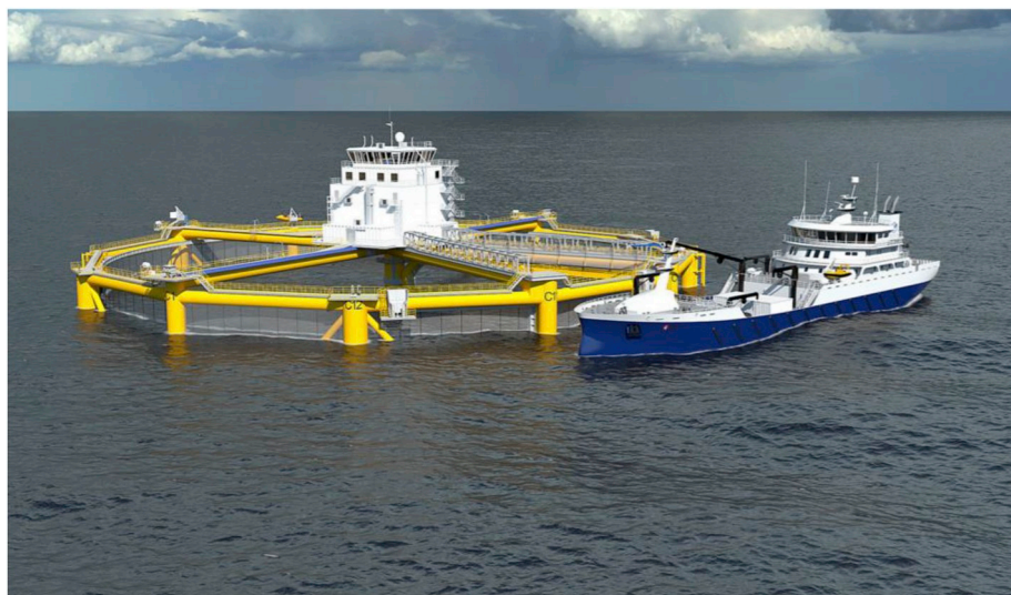
Fig. 1. Illustration of the ocean farming concept 'OCEAN FARM 1', illustration by Global Maritime.
