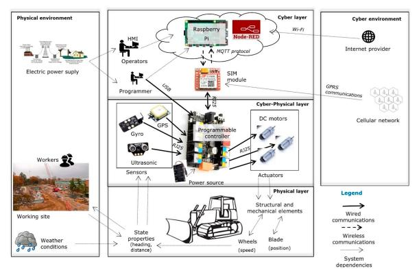
Figure 2. System representation as multi-layered CPS and environments.
