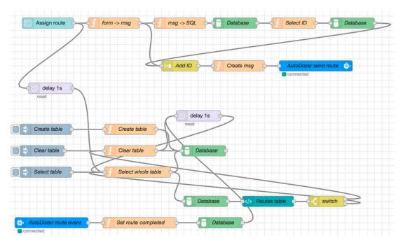
Figure 5. Flow diagram for route assignment in cloud platform.
