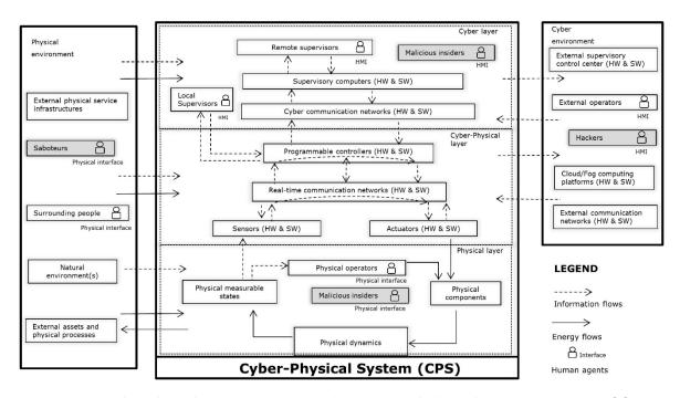
Figure 1. Cyber-physical systems (CPS) master diagram as multi-layered system representation [1].
