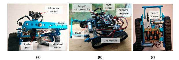
Figure 3. Prototype main views and parts explained (a) Front view; (b) left side view; (c) bottom view.
