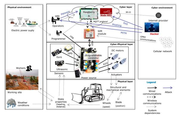
Figure 7. Mapping of threat actors and cyber–physical attack surfaces in CPS master diagram.
