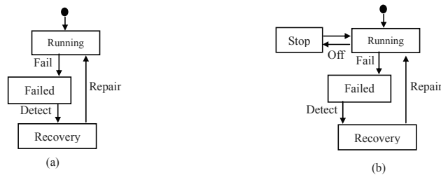
Figure 4(a). STM of software process (b). STM of hardware component
