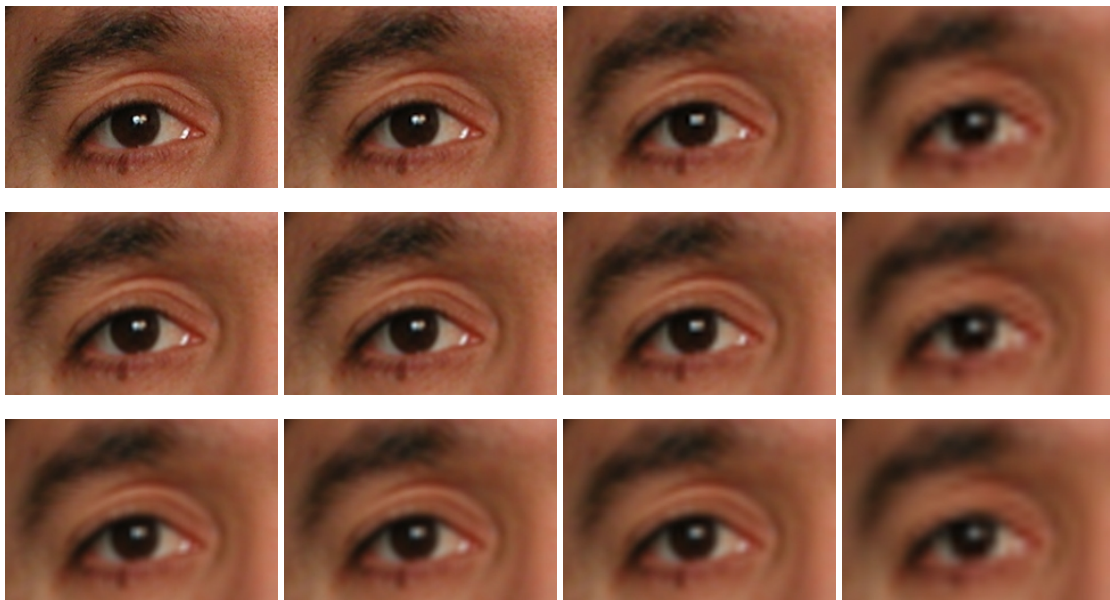
Figure F.8: Sample images from the test image on the left in Figure F.4. The top, middle and bottom row refers to blur index 0.24947, 0.42999, and 0.60378, respectively. The left column presents original test images with initial blur, while the rest columns to the right are the results with DF equals 2.0, 4.0, and 8.0, respectively. Images are to be seen on screen for best quality.
