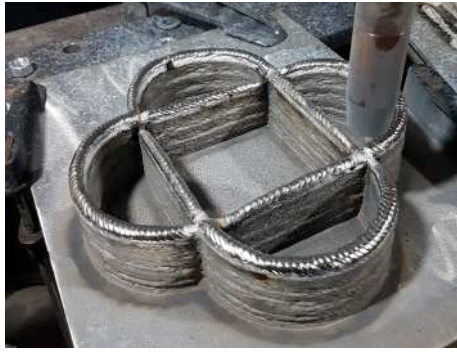
Fig. 7. Pulsed MIG: The final flower structure built in aluminium AA4043. This build has 65 layers, and some grinding was performed to reduce material accumulation in the intersections.
