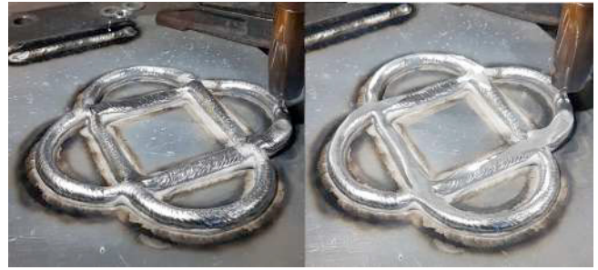
Fig. 11. Grinding: In the last test with aluminium AA4043 (fig. 7) some grinding was done every 10 layers or so in an attempt to avoid material accumulation in the intersection points.
