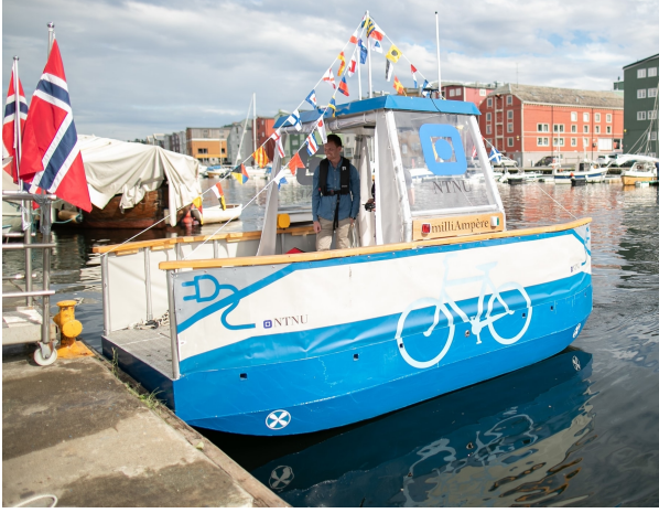
Fig. 1. The NTNU-developed, fully electric passenger ferry prototype, milliAmpere, used in the experimental testing. Photo: Kai T. Dragland
