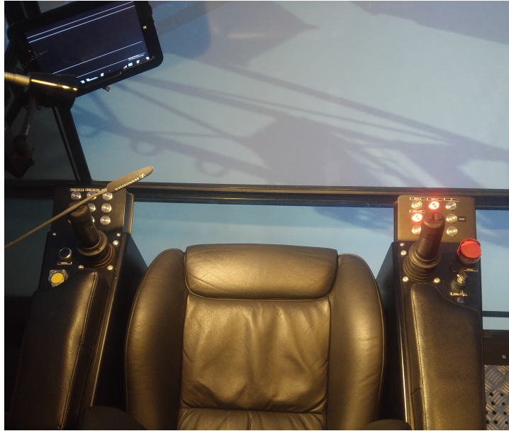
Figure 2.12: An operator chair as seen from above. Note the controls on each armrest and an alarm system tablet mounted to left. Picture was taken at OSC.
