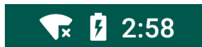
Figure 3.5: A symbol in the notification bar of an Android device letting the user know that it is connected to WiFi, but no Internet connection can be made.
