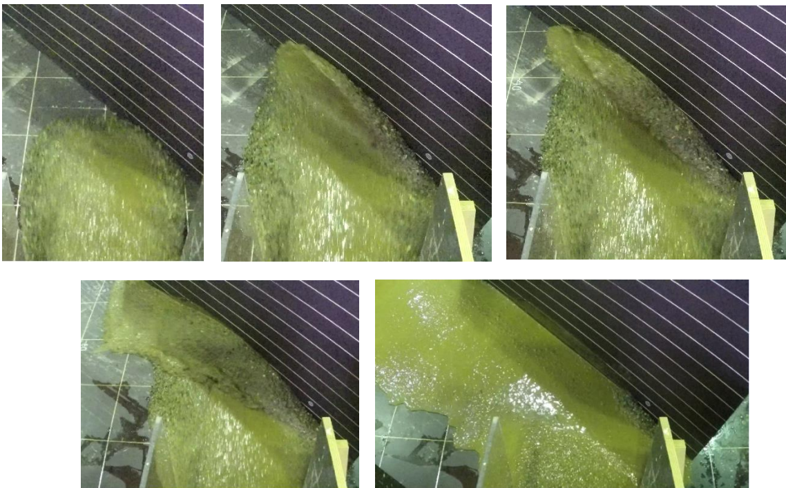
Figure 39: Upper left: Collision into the deflection wall, middle and upper left: upward splash and movement along the wall. Lower left: creation of a new front, lower right: height after the event (screenshot of test nr. 6 from Tracker).
