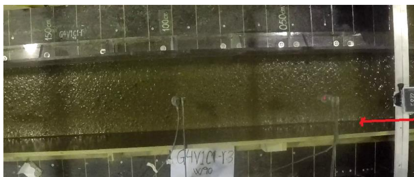
Figure 54: Accumulation of debris flow material in the chute in test nr. 11
