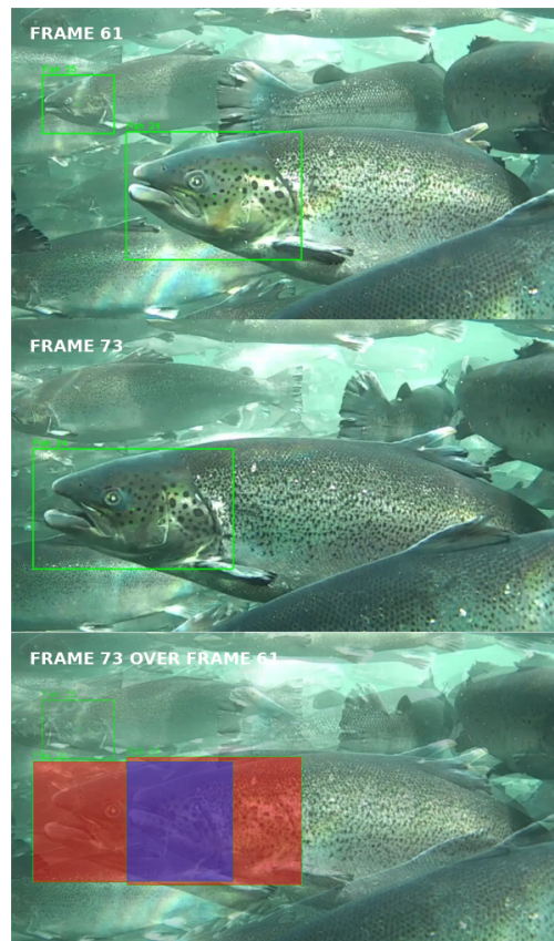
Figure 3.3: Illustration of IOU. The top image is frame 61 in the video, the middle is from frame 73, and the bottom image shows the two images over each other. Despite being 12 frames apart, the IOU is still quite high. The red and blue area is the union between the bounding boxes, and the blue area alone is the intersection.
