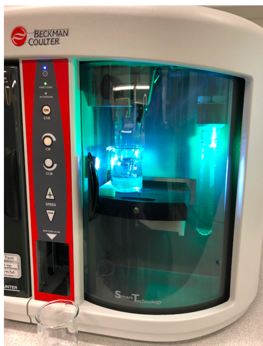
Figure A.1.6: Trying to count the plastic particles with the Beckman Coulter
