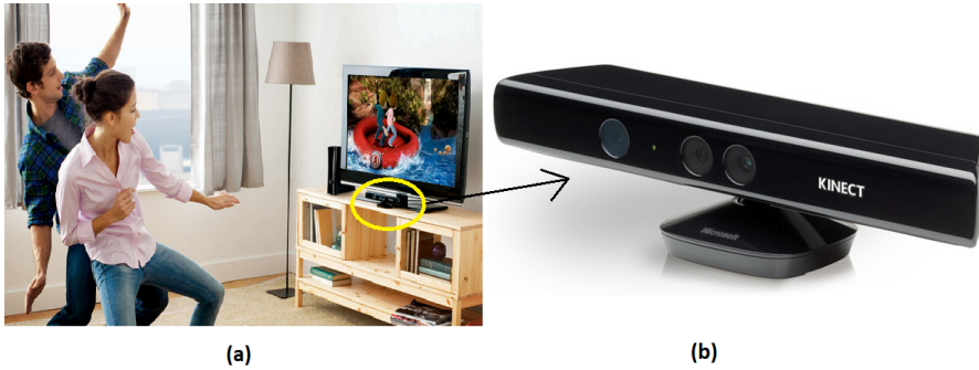
Figure 4.1: The Kinect sensor (a) together with the rest of the needed equipments, and (b) alone
