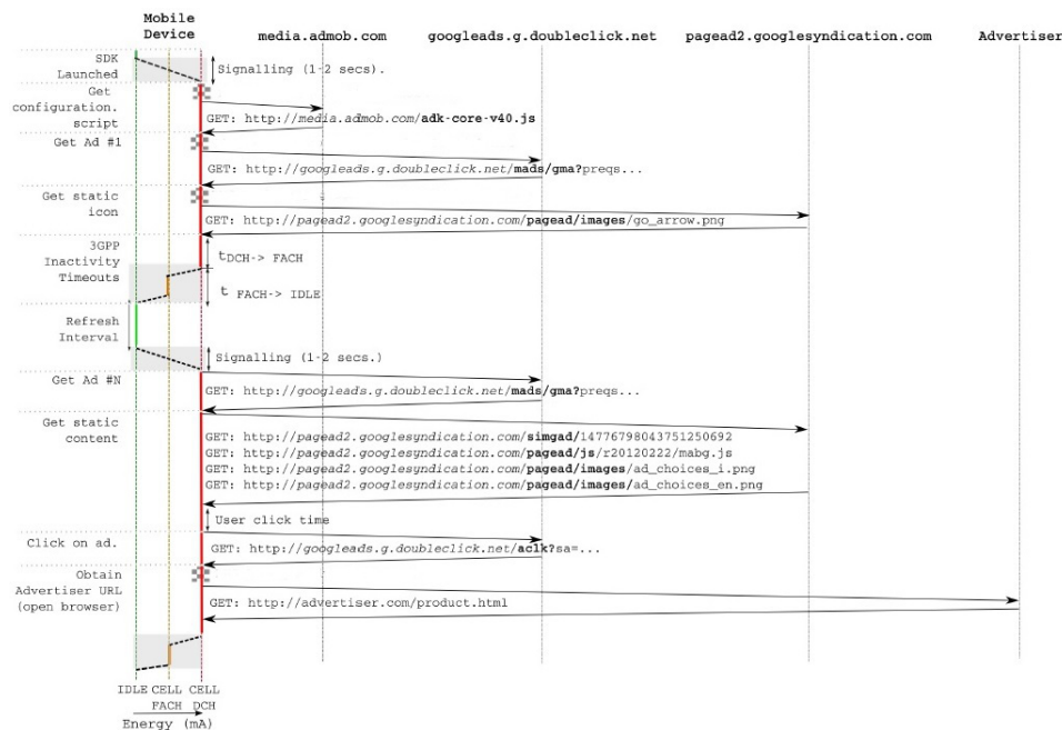
Figure 2.7: HTTP communication between a mobile device and Ad Network's servers for advertisement delivery. Modified from [37]
