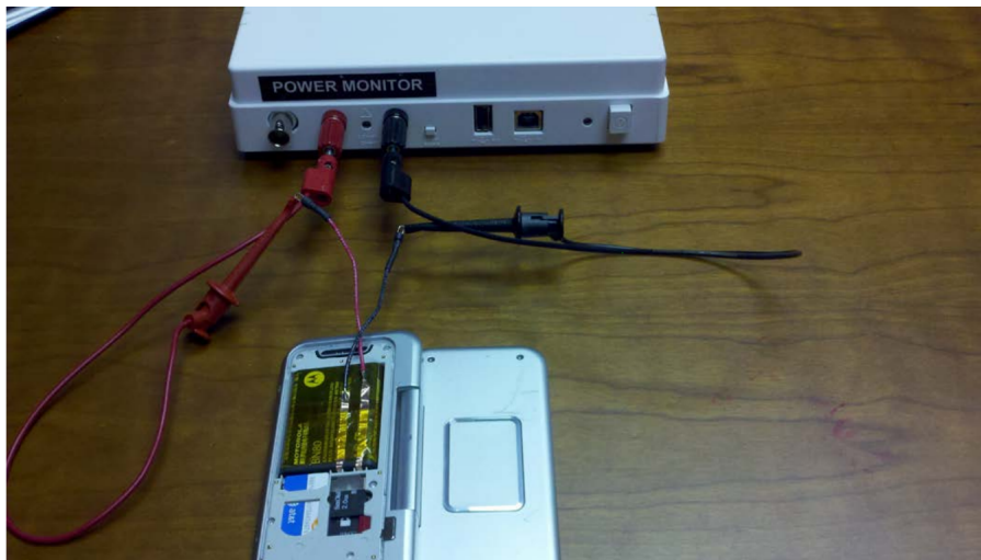
Figure 5.2: Power Monitor hardware device connected to a mobile phone to measure energy consumption. Taken from [20]
