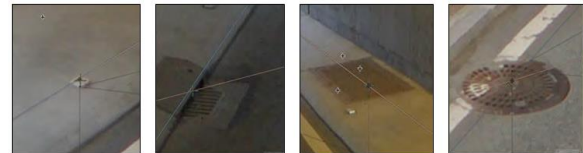
Figure 3: Sample examples of object types used in the measurement campaign (lamp, reflector mark, storm drain, manhole).
