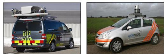
Figure 1: Left: Optech Lynx Mobile Mapper system installed on a vehicle. Right: Cyclomedia mobile mapping system Cyclomedia Technology B.V. (2010); Applanix (2014).
