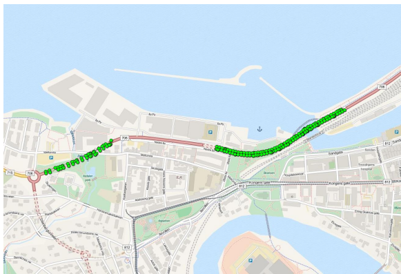
Figure 2: Trajectory and positions of the reference solution measurements (green circles) inside Ilsvik and Skansen tunnels, obtained by using total station equipment. Data collection performed by Nidaros oppmåling AS.
