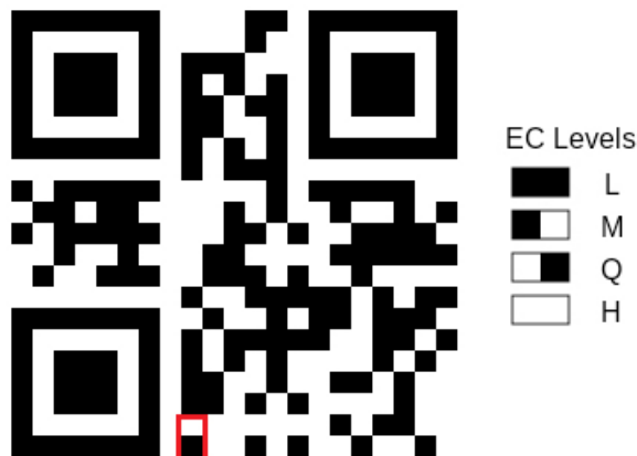
Figure 2.2: Error correction level of QR Code
