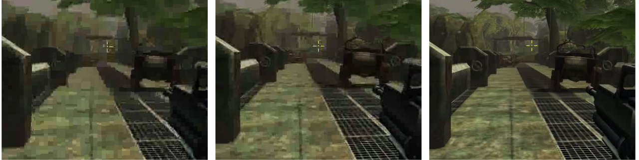
Figure 5.3: The effects of compressing a video stream of FarCry with WMV8 and three different video bitrates: 512 Kbps (left), 1 Mbps (middle), and 3 Mbps (right)
