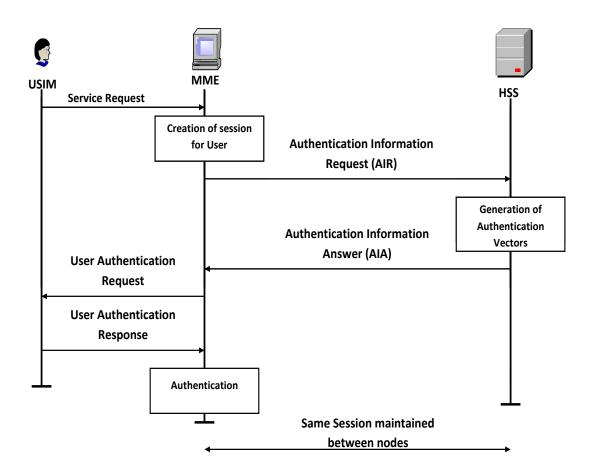
Figure 2.11: Application of Diameter for AKA process.
