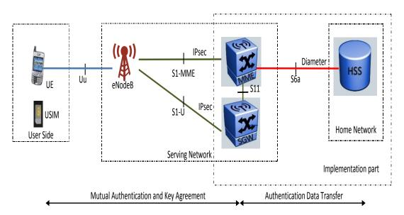
Figure 2.1: LTE Security Architecture with Interfaces.
