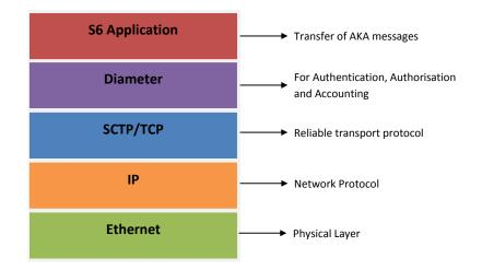
Figure 4.1: The S6 Protocol Stack (modified from [43, 49]).
