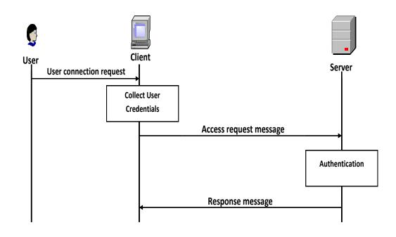
Figure 2.9: General Message Diagram for Diameter Authentication.
