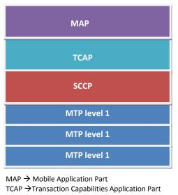
TCAP → Transaction Capabilities Application Part SCCP → Signalling Connection Control Part MTP → Message Transfer Part
