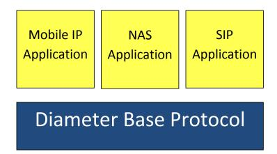
Figure 2.7: The Diameter Applications on top of Diameter Base Protocol [40].
