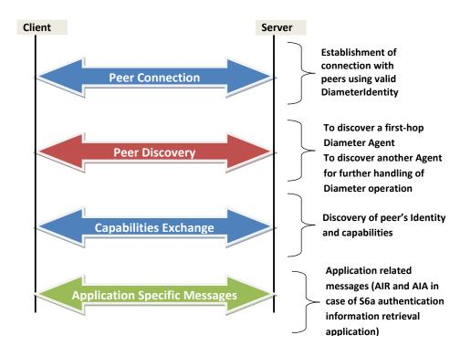
Figure 2.10: Diameter Message Exchange.
