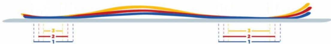
Figure 2.5: Ski curvature for cold conditions (blue), medium conditions (red), and warm/soft conditions (yellow)[5]
