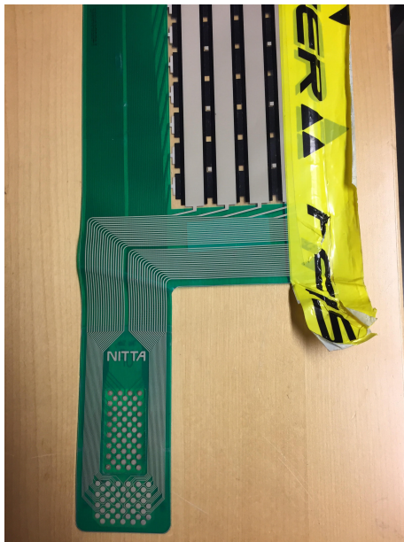
Figure 3.4: Pressure mat used by OLT
