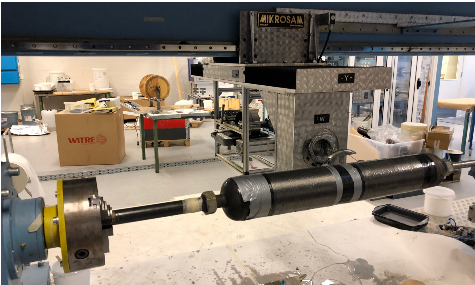
Figure 3.1: MicroSam automated filament winding machine during production of composite tubes.
