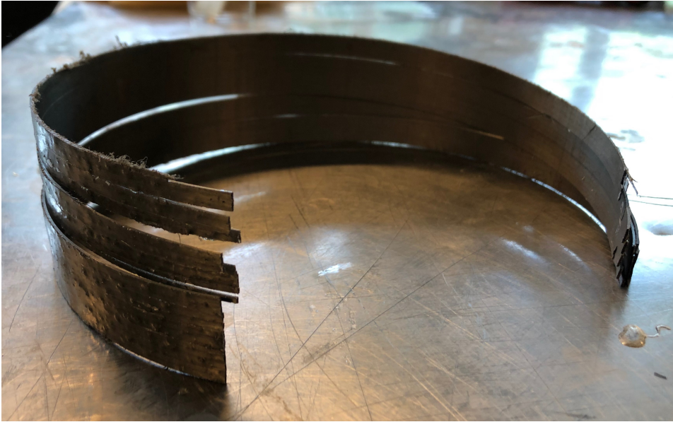
Figure 5.3: SFRP ring specimen after split-disk test.
