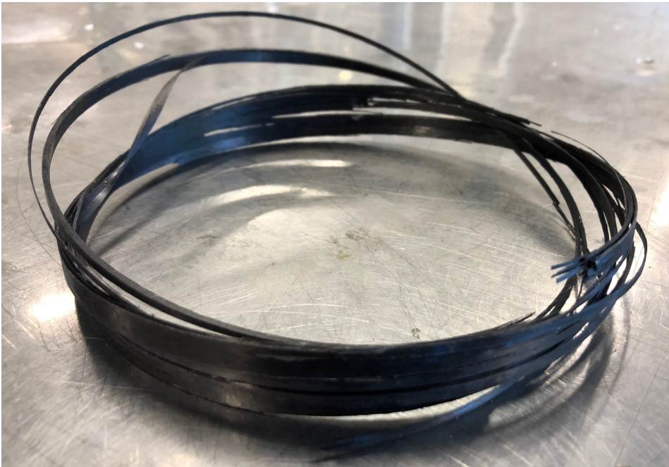
Figure 5.5: Broken CFRP ring specimen
