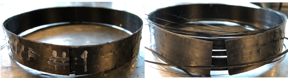
Figure 5.4: Broken hybrid samples. To the left: hybrid sample with first-ply-failure in SFRP layers. To the right: hybrid samples that experienced ultimate fiber failure
