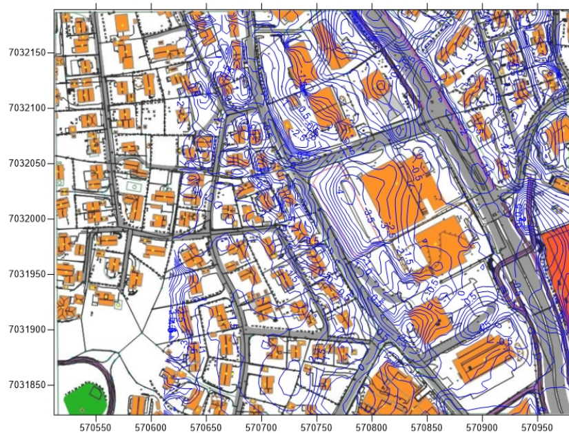
Figure 2.6: Change in ground level between 1951 and 2018
