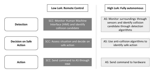
Figure 7: High level tasks for low and high Levels of Autonomy
