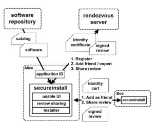
Figure E.4.: System Architecture. The prototype was implemented on the Nokia N810 tablet, while a rendezvous server was setup on an Ubuntu desktop. The prototype interacts with conventional software repositories to obtain application catalog and installation packages.
