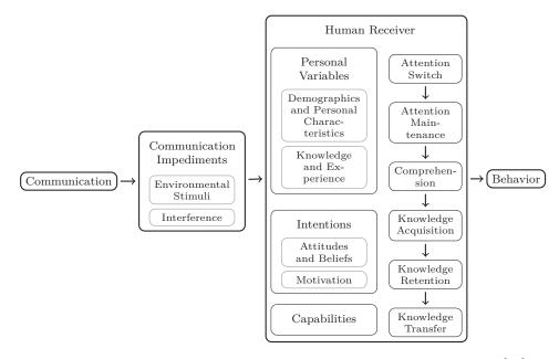
Figure 1.1.: The human-in-the-loop security framework provided by Cranor [44] for reasoning about the cause of security failures attributable to human errors.
