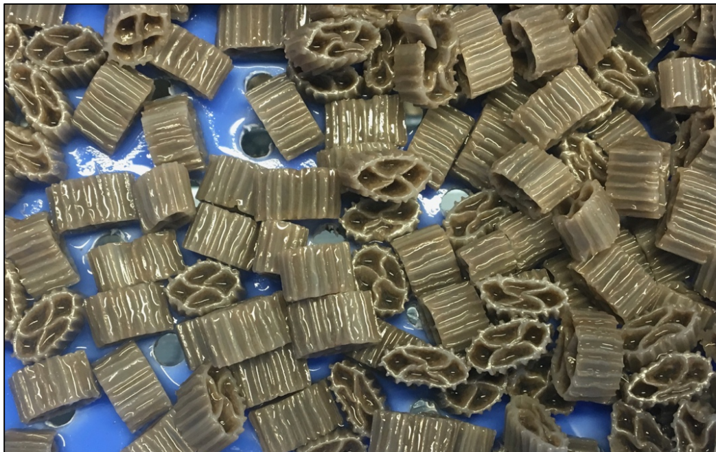
Figure 3.6 Carriers in CMBBR with biofilm attached
