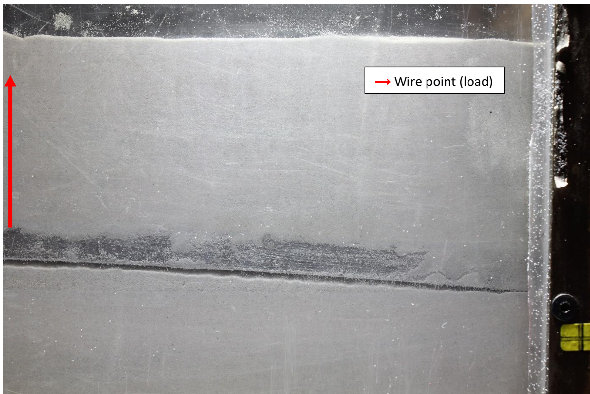
Figure 61: Pipeline deflection at the last image taken before failure. It is difficult to say if rotation occurs at the end of the pipe, but it is entirely plausible that the ends are still fixed. Also note that sand is falling into the gap between the pipe and the window.
