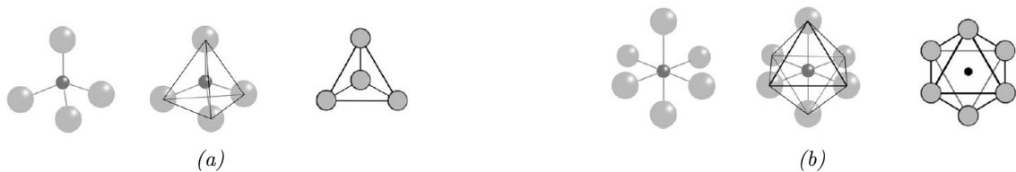
Figure 2.13: Ball-and-stick models and polyhedral models for tetrahedra (a) and octahedra (b) molecular structures [4]
