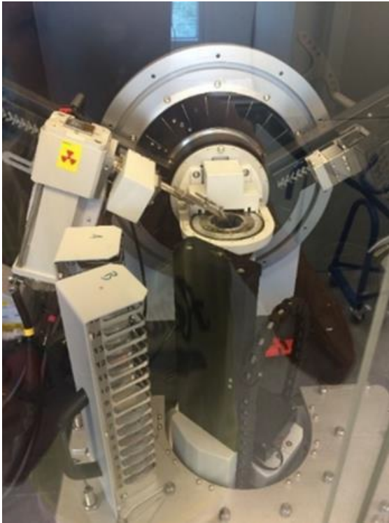
Figure 3.1: XRD apparatus used at NTNU labs [31]
