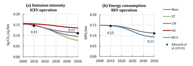
Figure 3.4a-b – Parameters for the emissions intensity of ICEV operation and energy consumption during BEV operation, shown in kilo CO<sub>2</sub>-eqivalents and kWh per kilometer, respectively.
