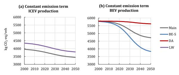
Figure 3.2a-b – Constant emission parameter for producing the ICEV and BEV, given in kilo CO<sub>2</sub>-equivalents per vehicle produced. The chart for the ICEV is shown in the main and the light-weighting (LW) scenarios, while the chart for the BEV is showing the main, battery electric success (BE-S) and delayed action (DA) scenarios.
