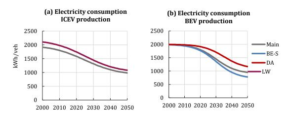
Figure 3.1a-b – Electricity requirement of producing the ICEV and BEV shown in kWh per vehicle produced. The chart for the ICEV is showing the main and light-weighting (LW) scenarios, while the chart for the BEV is showing the main, battery electric success (BE-S) and delayed action (DA) scenarios.
