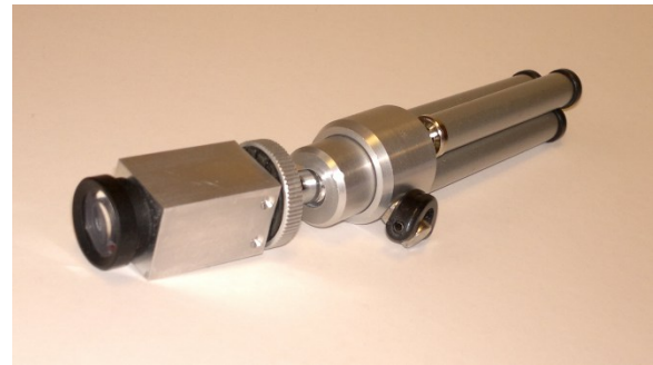
Figure 8. The Camera Module assembled, using a mechanical positioning system. The size of house with lens is approx. 17 x 17 x 38 mm.
