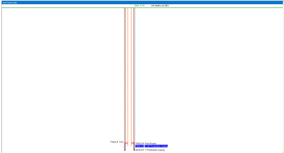
Figure 4.1: Well schematic showing the production packer, tubing and casing setting depth and TOC for well "X"
