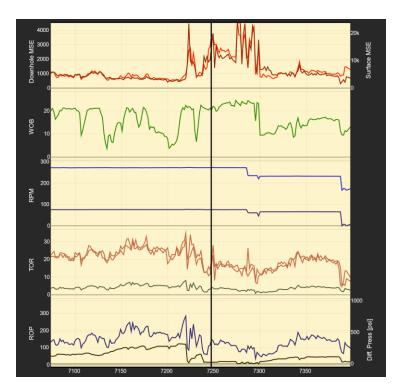
Figure 5.3: Bit balling response seen in what is most likely a shaly part of the Gemini Sand in the transition from the upper to middle zone. The interval is taken from the 12 1/4" section of well C4.
