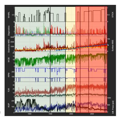
Figure 4.23: Damaging stringer detected, indicated by red fill.
