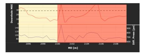
Figure 4.24: Differential pressure spiking along with MSE, i.e. typical stringer response.
