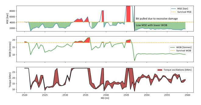
Figure 4.16: Stickslip scenario from well A3 with a bit trip on the black line. Stickslip events colored in red.
