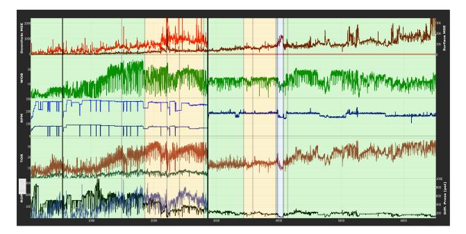
Figure 4.3: Well C4 Overview. Abrupt change in parameters when casing is set (Black vertical line).
