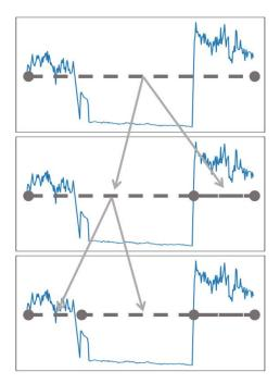
Figure 2.5: Binary segmentation method visualized. Segmentation performed according to magnitude of change.
