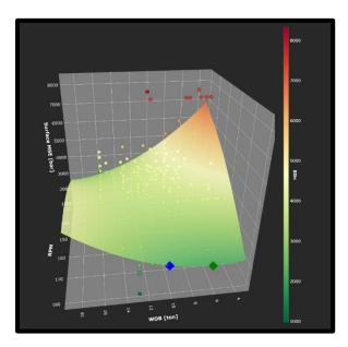
Figure 4.9: Surface generated from aggregated data points. Optimum located at blue point, minimum MSE at green point.
