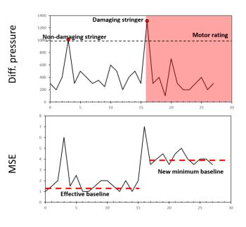
Figure 3.21: Stringer detection and damage assessment scheme overview
