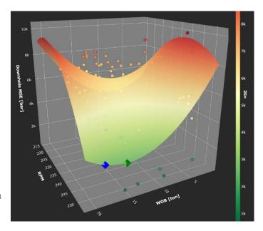
Figure 4.12: Generated surface from bent motor drilling. Optimal point in blue, minimum in green.
