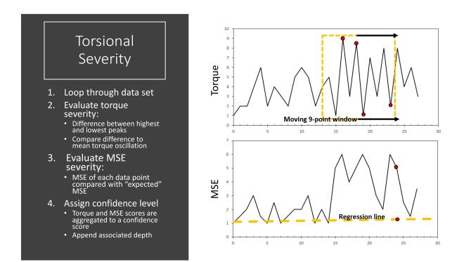
Figure 3.20: Torsional severity diagnostics overview
