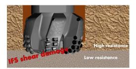
Figure 4.25: High load on bit shoulder in transition between laminated layers when exiting stringer.
