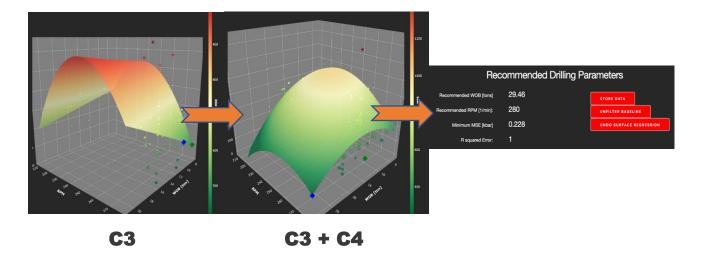
Figure 4.6: Introducing additional data points results in more accurate surface regressions, but also heavier computations. Output parameters are displayed together with recommended parameters.
