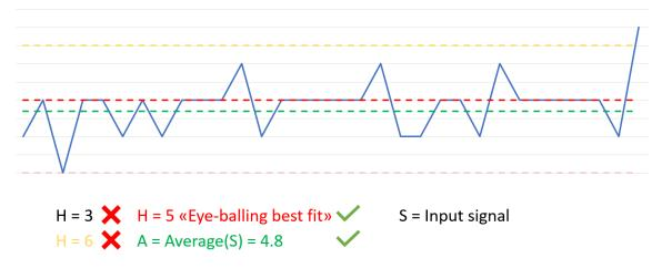
Figure 2.2: Example of different straight-line fits to an input signal
