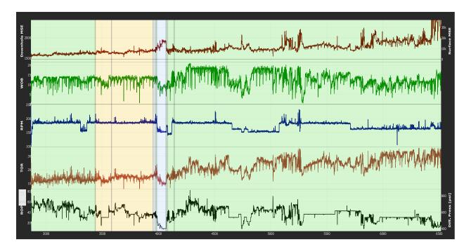
Figure 4.4: Well C4 8.5 Section, shale in green, sand in yellow and chalk in blue.
