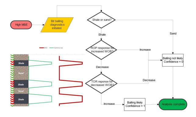
Figure 5.4: Proposed bit balling diagnostics procedure.
