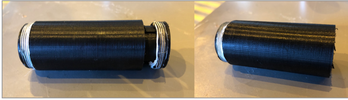
Figure 7.22: Plastic housing thread failure.
