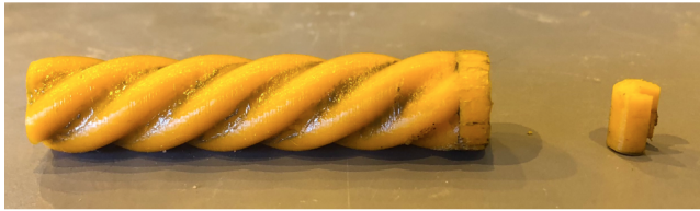
Figure 7.23: Rotor coupling failure.
