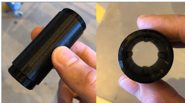
Figure 7.18: Modular design showing the outer plastic housing that holds the stator inside. Notice the splines inside the housing that take up the torque induced in the stator.
