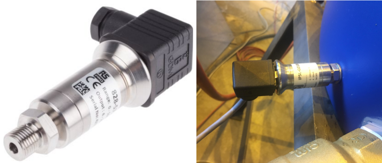
Figure 9.15: Pressure (level) sensor installed on the tank
