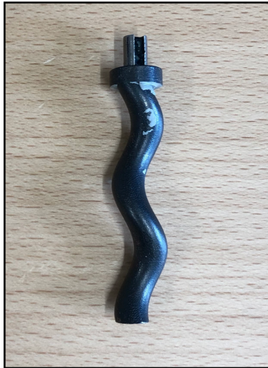
Figure 7.16: Peeled off rotor after a run inside the stator.
