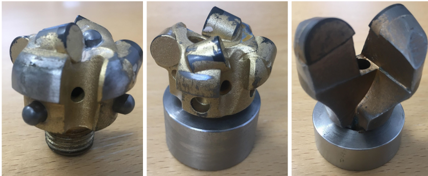
Figure 11.16: Tested bits (DSATS bit with inserts on right, without inserts in the center and Alibaba bit on the right)
