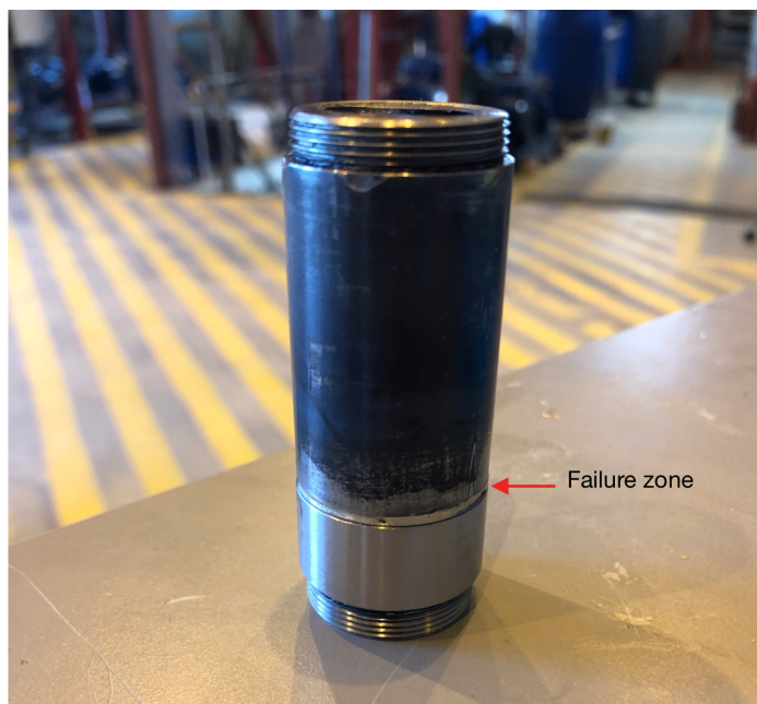
Figure 7.17: Repaired stator after a brittle failure in the threaded zone.
