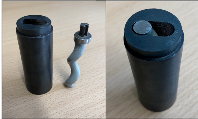
Figure 7.15: Steel rotor and stator.
