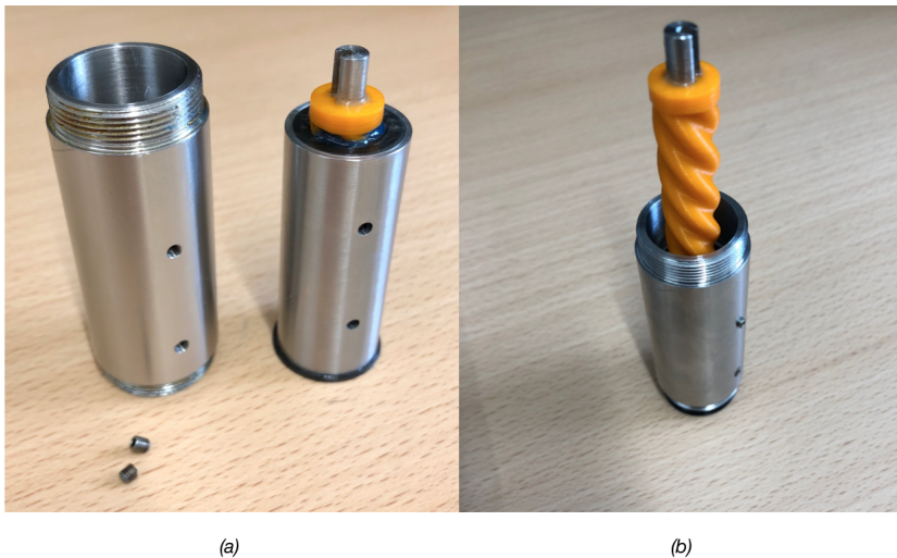
Figure 7.25: New power section assembly. (a) The inner sleeve can be retrieved and replaced without affecting the outer housing. (b) Power section ready to be used.
