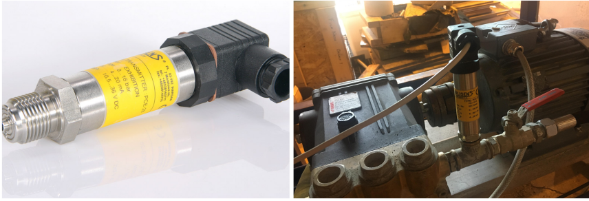
Figure 9.13: Pressure sensor installed on the rig
