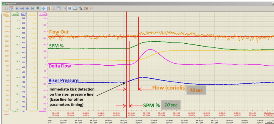
Figure 2.9: Immediate kick detection during kick drill with the use of CML technology (Elahifar et al., 2017).
