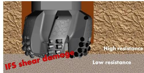
Figure 4.25: High load on bit shoulder in transition between laminated layers when exiting stringer.
