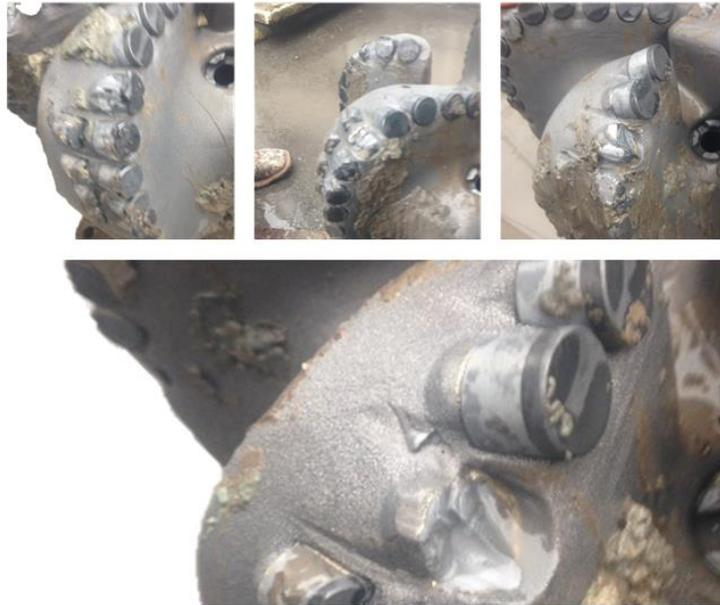
Figure 4.22: Bit pictures with clear IFS damage.
